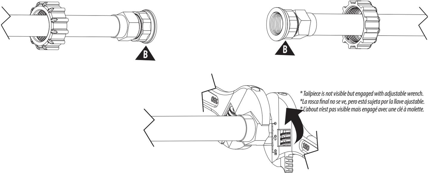
\* Tailpiece is not visible but engaged with adjustable wrench.
