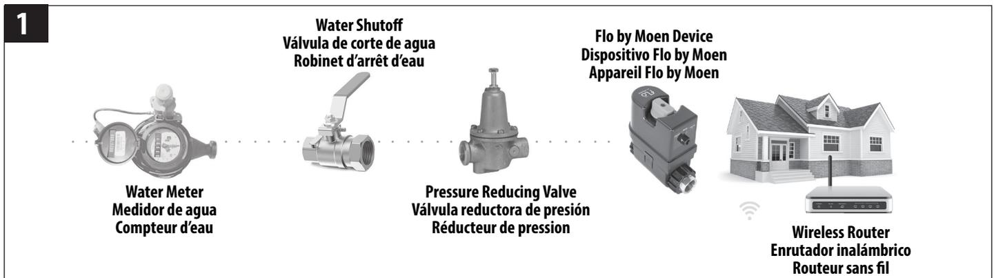
Determine the best location for the installation spacer kit and future Flo by Moen Smart Water Shutoff.
