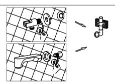
8. Warp the thread of spout with teflon tape (ensure it must warp clockwise). Screw-in to the inlet pipe inside the wall, then install the decorative cover on the wall clingy.
