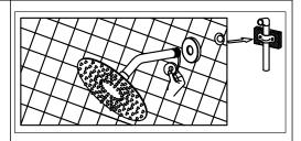
9. Install the shower arm, shower head and flange to the fitting. (stick to the wall) . Tighten the showerhead to the shower arm with the pipe tape (Make sure the pipe tape with clockwise direction).
