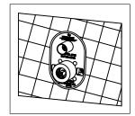
4. Please cut the size of the tile hole according to the size and shape of the protetived cover ( about 5mm bigger than the protetived cover from each side ) . And please put the tile outside the wooden wall ( please noted that we keep the same central point for the tile hole with the protetived cover ) .
