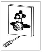
1. Confirm the installed place of the pressure balance valve and fixed on the wood block.
