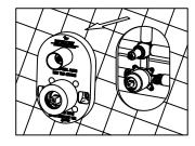
5. Loosen the screw and remove protect cover.
