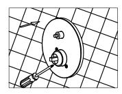
6.Lock the deck plate into the body and cling to the wall, then tight the screw.
