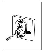
3. Lock the install protective cover into the body. ( 155\*100mm oval type).
