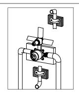
2. Connect the hot&cold inlet tube and outlet tube, then make sure the tube fix stable on the wooden wall.
