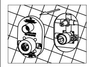
5. Loosen the screw and remove protect cover.
