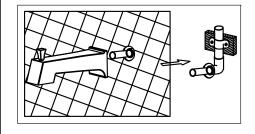
11. Insert the spout to the pipe which outside the wall, then tighten the screw.
