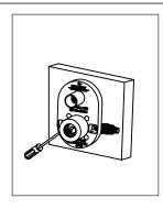
3. Lock the install protective cover into the body. ( 155\*100mm oval type).
