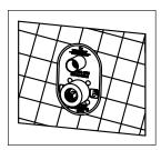
4. Please cut the size of the tile hole according to the size and shape of the protetived cover ( about 5mm bigger than the protetived cover from each side ). And please put the tile outside the wooden wall ( please noted that we keep the same central point for the tile hole with the protetived cover ) .
