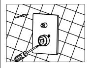
6.Lock the deck plate into the body and cling to the wall, then tight the screw.
