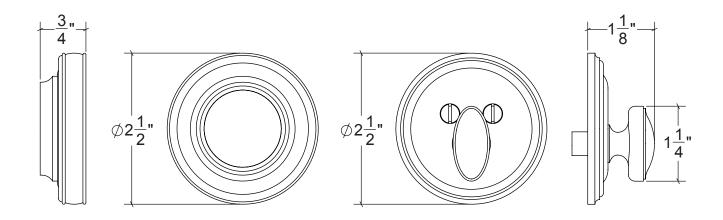
Works with door thickness 1-3/4" to 2-1/4" Works with 2-1/8" bore face
